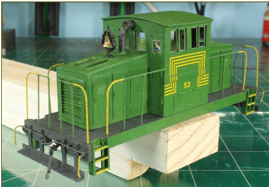
Figure 6 – The locomotive has been painted and decals added. Uncoupler levers and air hoses were added to the pilots. The bell on the hood came from an old steam locomotive.
